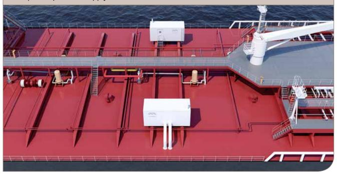
The technical teams for Alfa Laval ballast water treatment systems and Framo pumping systems have developed a solution for providing additional pumping head when PureBallast 3 Ex is installed in a deckhouse. By ensuring that the PureBallast 3 Ex system can handle its own pressure requirements, the optional booster pump unit (BPU) removes the need for changes in the existing ballast pumping system, thereby retaining its optimization and the vessel's cargo offloading rates.
